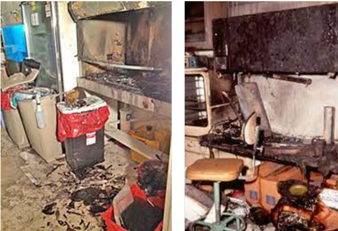
Figure 16. The results of a fire/explosion in a Biosafety Cabinet.
